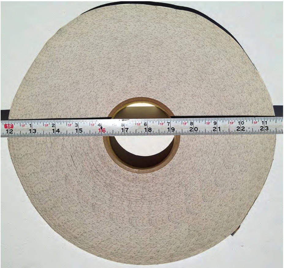
Figure 11. The diameter of the full 30,000-stamp coils of the 29¢ Eagle linerless self-adhesive imperforate test coil stamp is approximately 11¾ inches.
